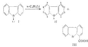
When one equivalent of *n*-butyllithium was used in the above reaction the result was a 56% recovery of dibenzothiophene-5-oxide, a 3.5% yield of diben zothiophene-4-carboxylic acid and a 4.4% yield of dibenzothiophene.
